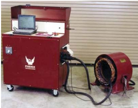
Core Loss Testers are available for testing from fractional to 16,000 HP motors.
